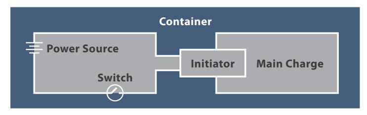
Multiple switches are sometimes present and connected together
